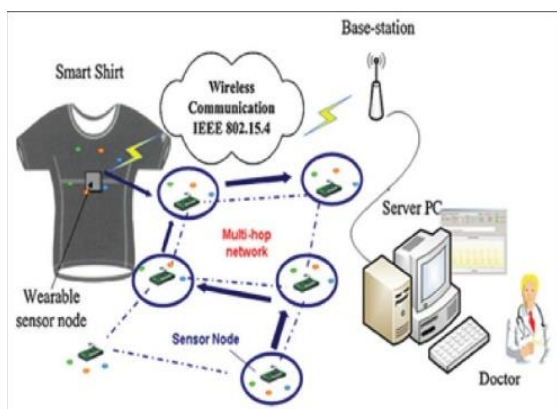
Figure 7: System Architecture with Smart shirt
