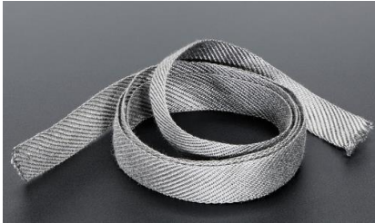
Figure 2: Electro conductive ribbon sample [42] Reprinted from http://www.titvgreiz.de , with permission of TITV Greiz.
