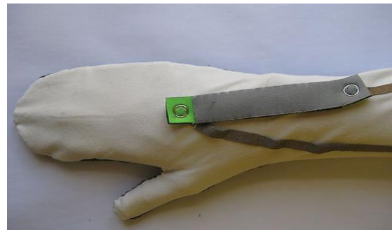
Figure 5: A textile bend sensor created is using conductive fabric and neoprene
